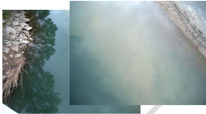
Figure 5 – Photographs taken from the upstream side of Road 94B Bridge showing the mixing zone of Gordon Slough and Cache Creek. Photos taken on April 19, 2004. At the time of the photo Cache Creek turbidity upstream of the confluence was 2.2 NTU (lab), while that of Gordon Slough was 62 NTU (lab). Photos only show a portion of the Gordon Slough effluent. More highly turbid water joined the creek ~100 yards downstream, downstream of the bridge. (Photos: Chris Hammersmark)
