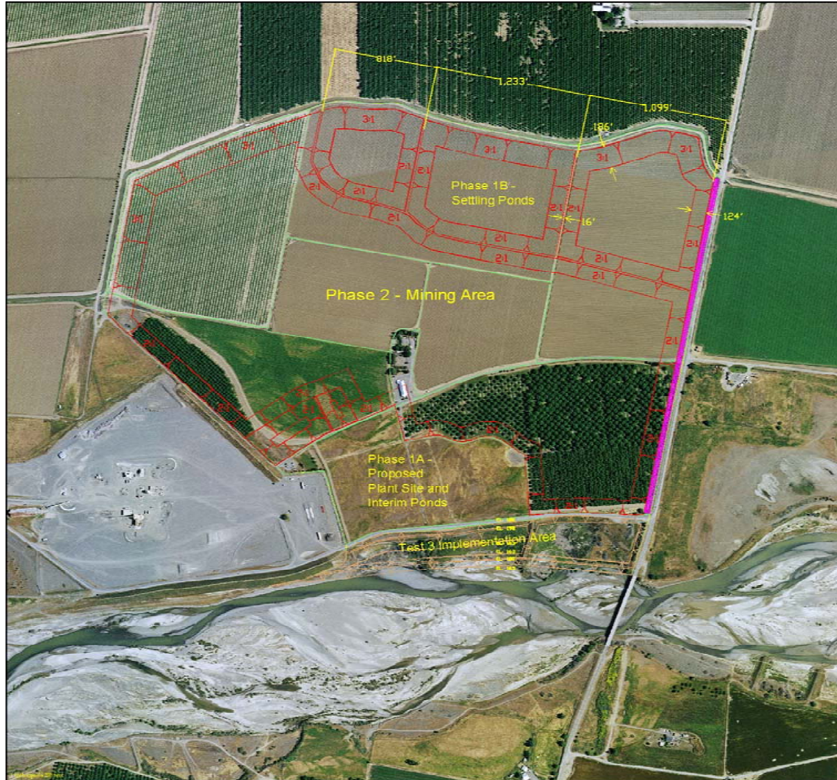
Figure 2 Project Boundaries and Phases Granite Esparto Plant
