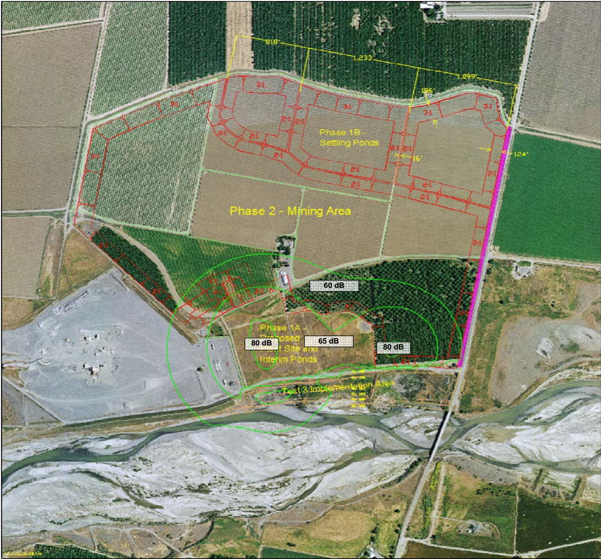
Figure 5 Hourly Average Noise Level (Leq) Contours Granite Esparto Plant Phase 2 Operations in Southeast Portion
