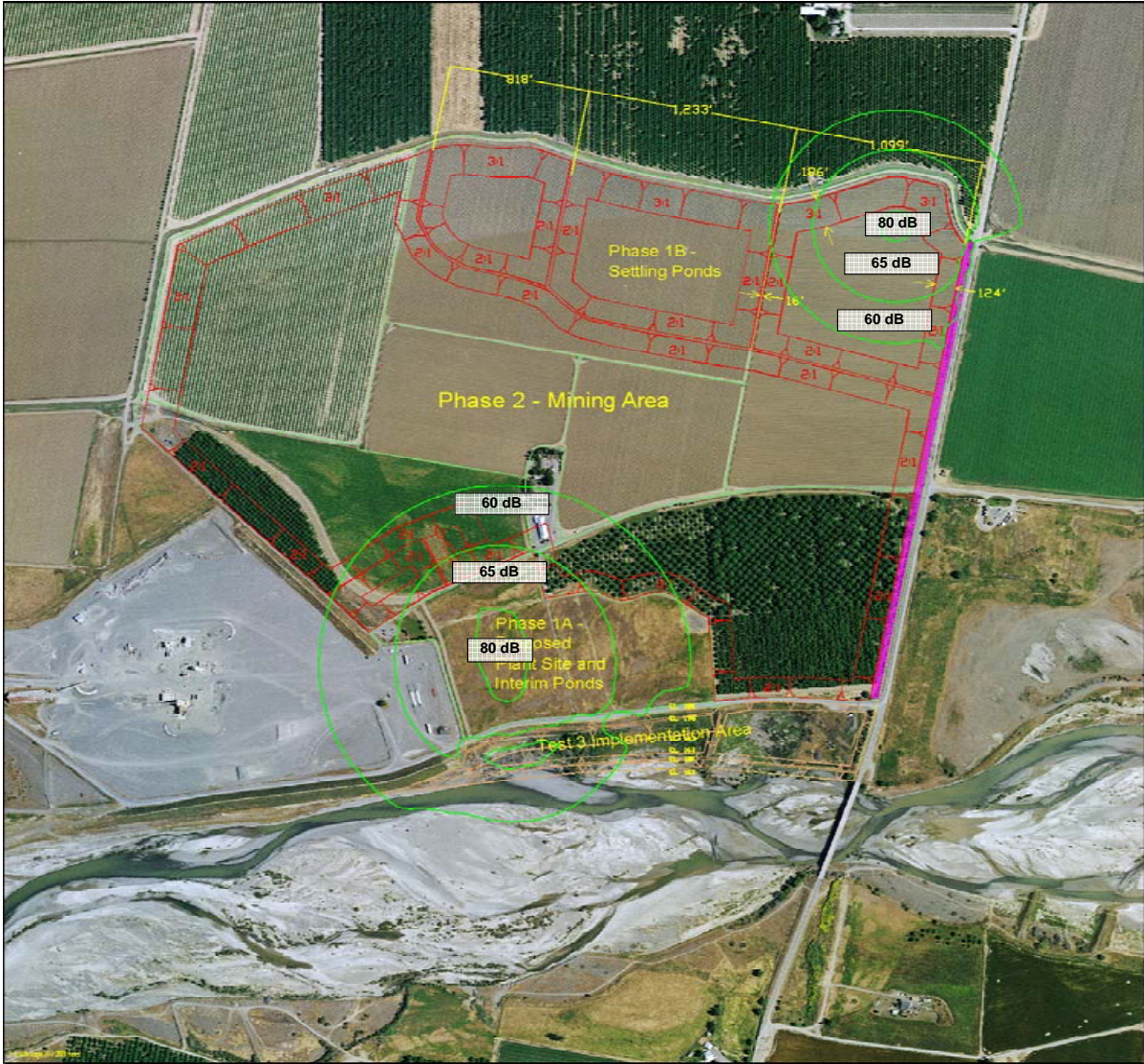
Figure 3 Hourly Average Noise Level (Leq) Contours Granite Esparto Plant Phase 1B Operations at Northeast Corner
