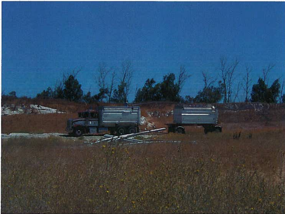
Semi-Truck operator is providing water to the load of lime chalk prior to exiting the project site.
