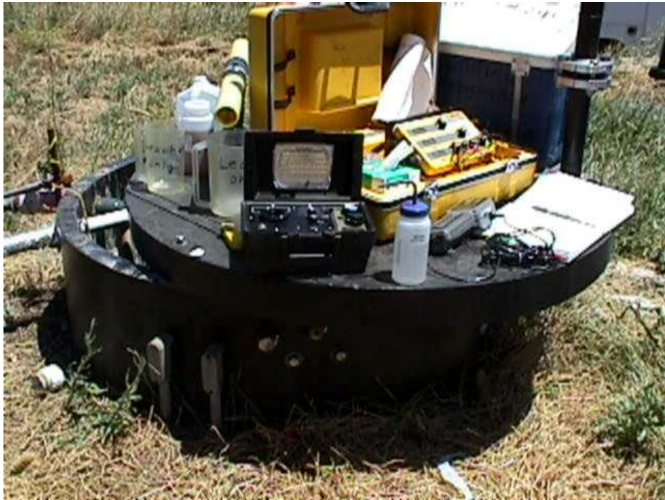
Figure 1. Field equipment used to take leachate field parameters.
