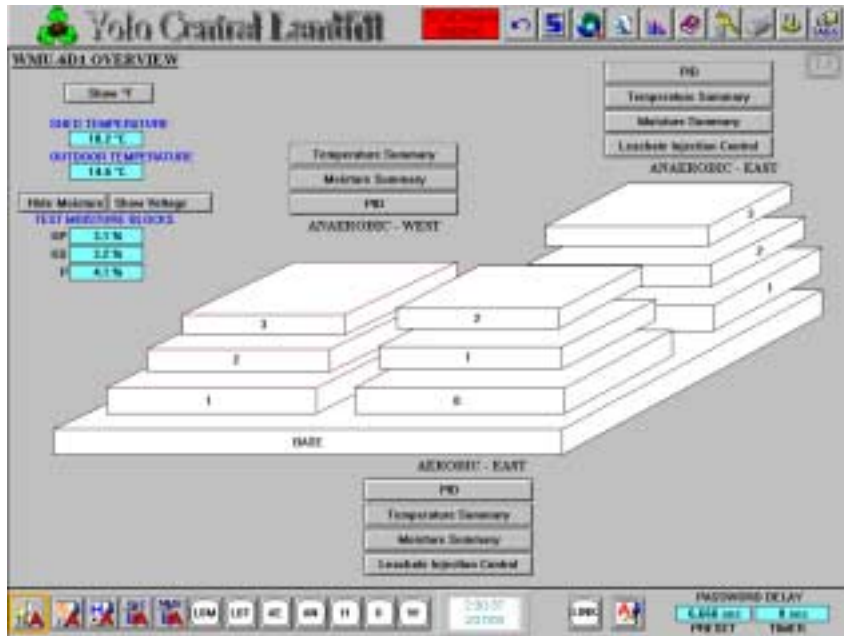
Image 4-2: SCADA overview screen. From here you can access each layer within the bioreactor cells.
