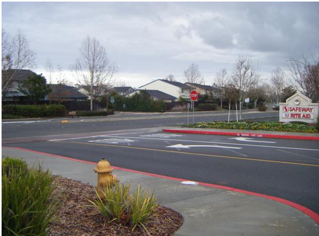
Figure 15: This parking lot entrance has low landscaping on both sides in order to maintain a clear line of sight. The sign is set back so that it does not obstruct visibility.
