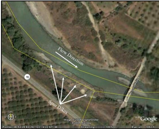
Existing Spur Dike Locations
