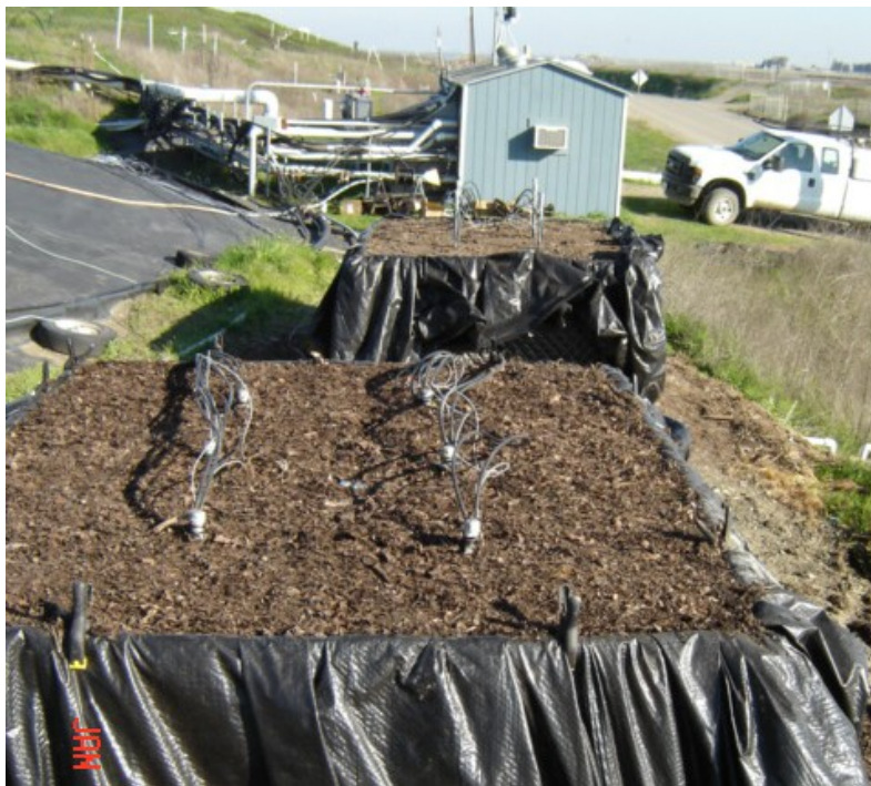
Figure 9. Cells completed. Tubing and wires for temperature sensors connected to instrument shed in background.
