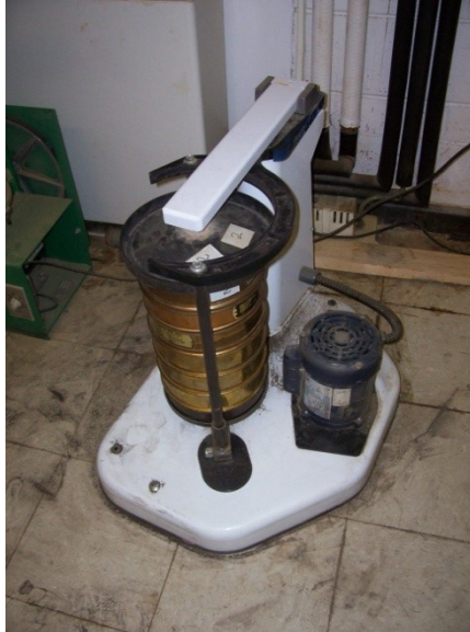
Figure 12. Shaker that was used to perform sieve analysis.
