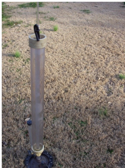
Figure 15. Tension disk infiltrometer used to perform infiltration test.
