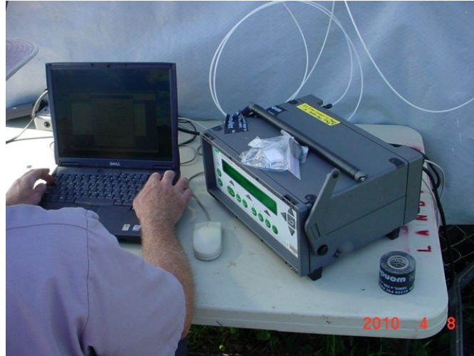
Figure 17. PAS (on right) used to measure SF 6 , CO 2 , and CH 4 in field for flux tests.
