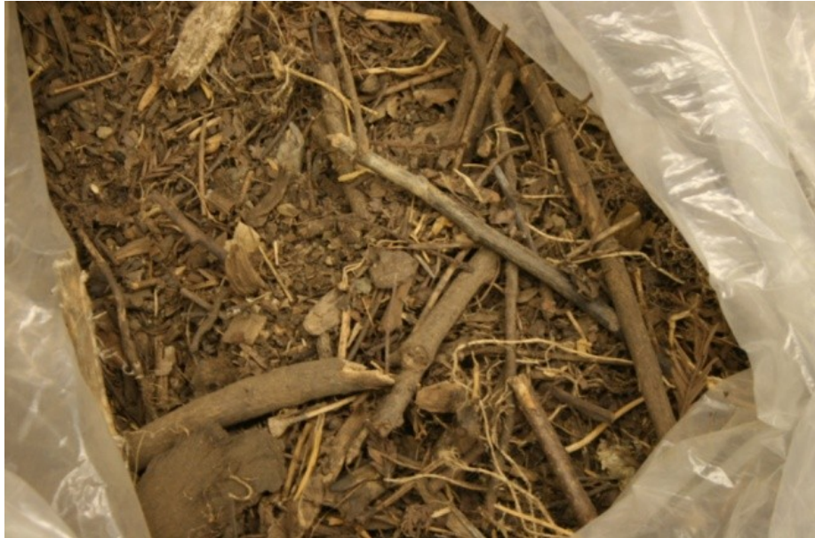
Figure 11. Fresh green material used to construct biocover #2.
