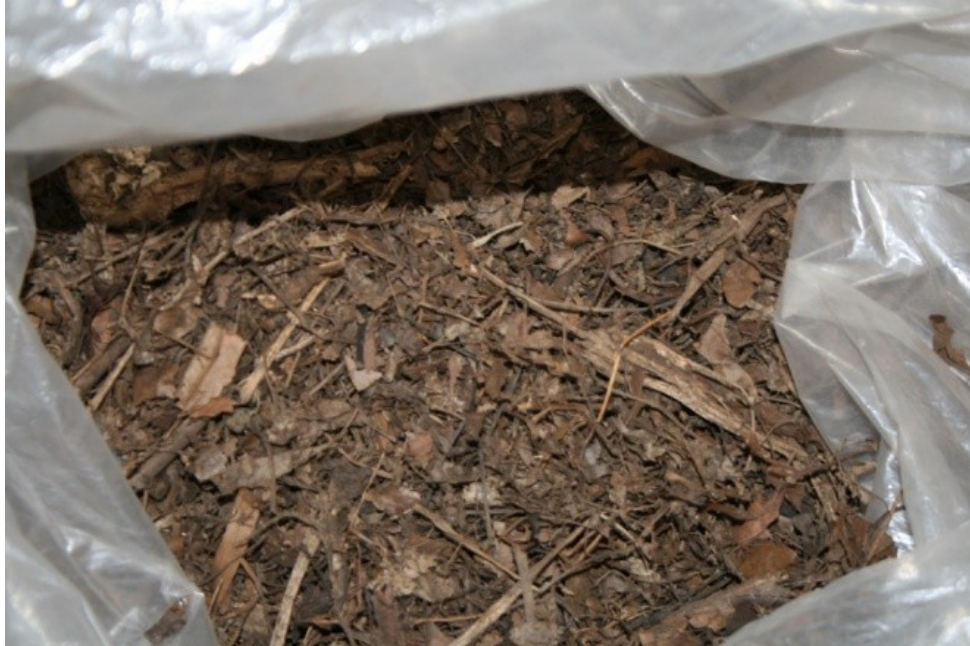
Figure 10. Aged green material used to construct biocover #1.
