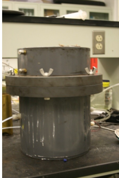
Figure 13. Experimental setup to measure gas diffusion coefficient.
