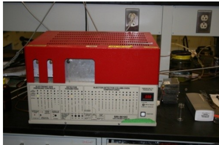
Figure 14. Gas chromatograph used to measure tracer gas concentration.
