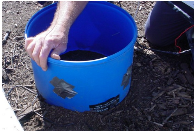
Figure 18. Small-scale flux chamber used to quantify the spatial variability of surface CH 4 fluxes from biocover test cells.
