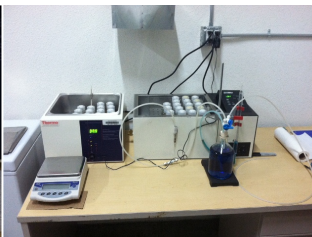
Figure 2. BMP digester setup with water bath temperature control and gas measurement.
