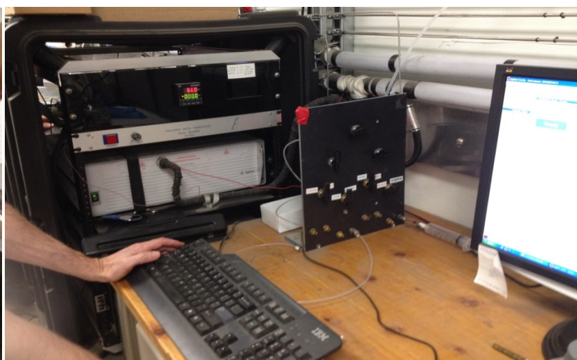
Figure 3. Gas sampling (left) and analysis (right) of BMP assays using gas chromatograph
