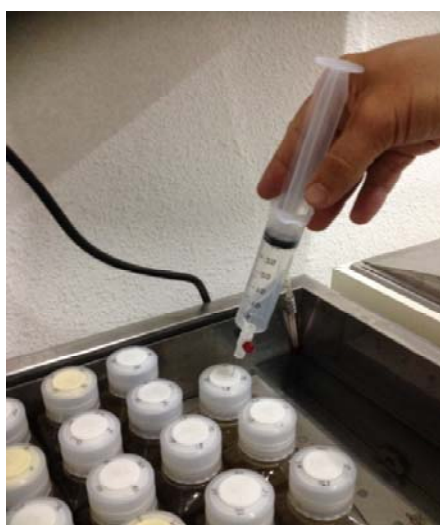
Figure 3. Gas sampling (left) and analysis (right) of BMP assays using gas chromatograph
