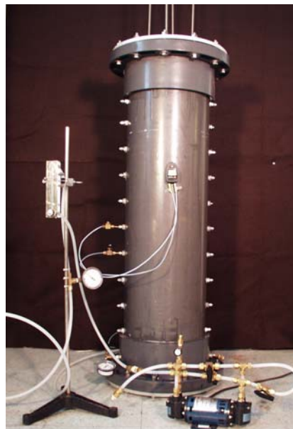
Figure 2-24. Photograph of experimental cell used for air permeability tests of biocover materials
