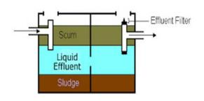
of the leach field and the soils, usually <u>every 3-5 years</u>; but the use of the system will determine how often the tank should be pumped. Washing machines, dishwashers, and garbage disposals will increase the amount of sludge, and the tank will require more frequent pumping.
