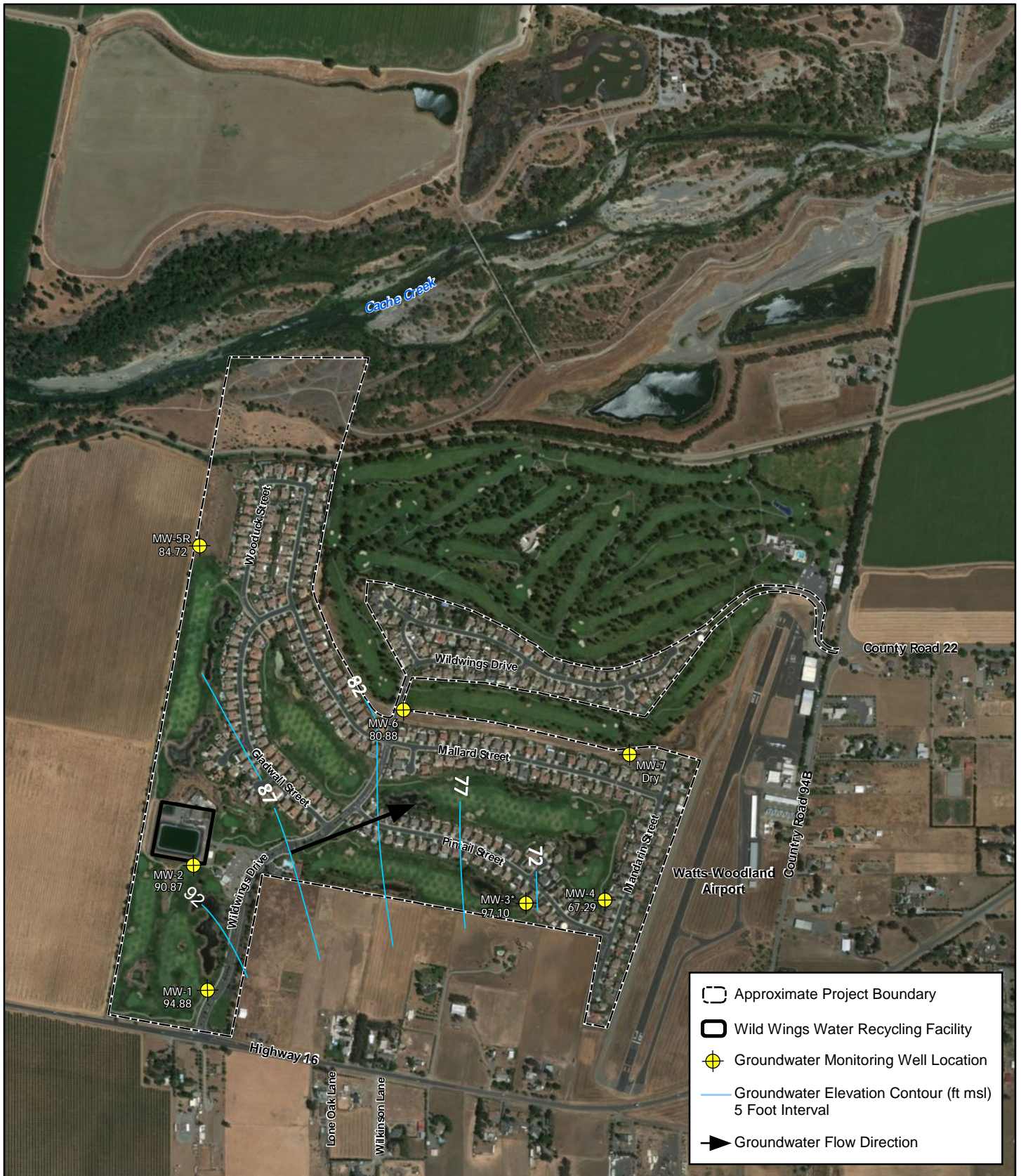
Figure 2 Groundwater Elevation Contours
