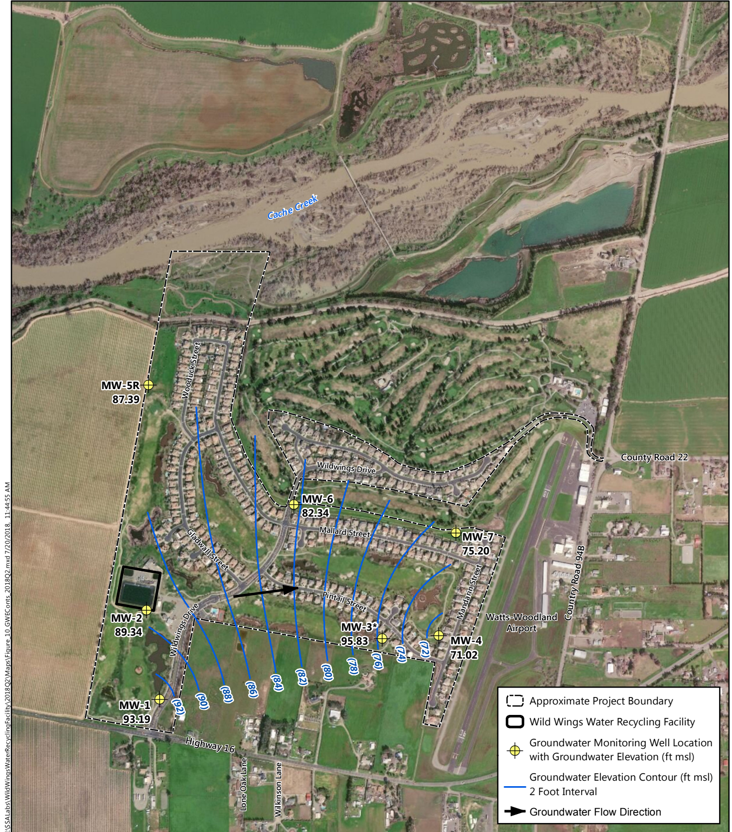
Figure 10 Groundwater Elevation Contours Second Quarter 2018 Monitoring Report Wild Wings Water Recycling Facility 18530 Wildwings Drive Woodland, Yolo County, California
