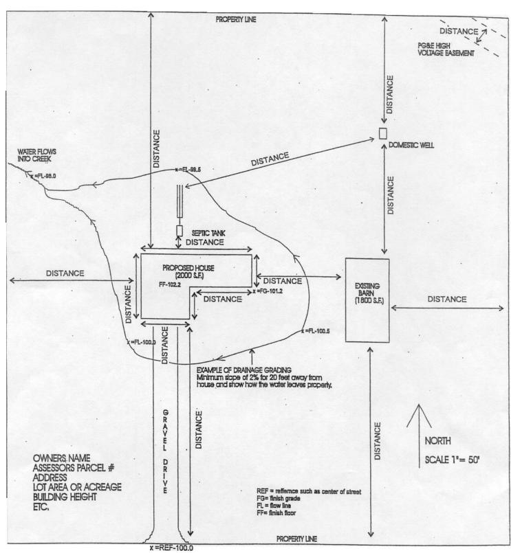
(without a true survey a point is picked as the reference elevation as the center of the street)
