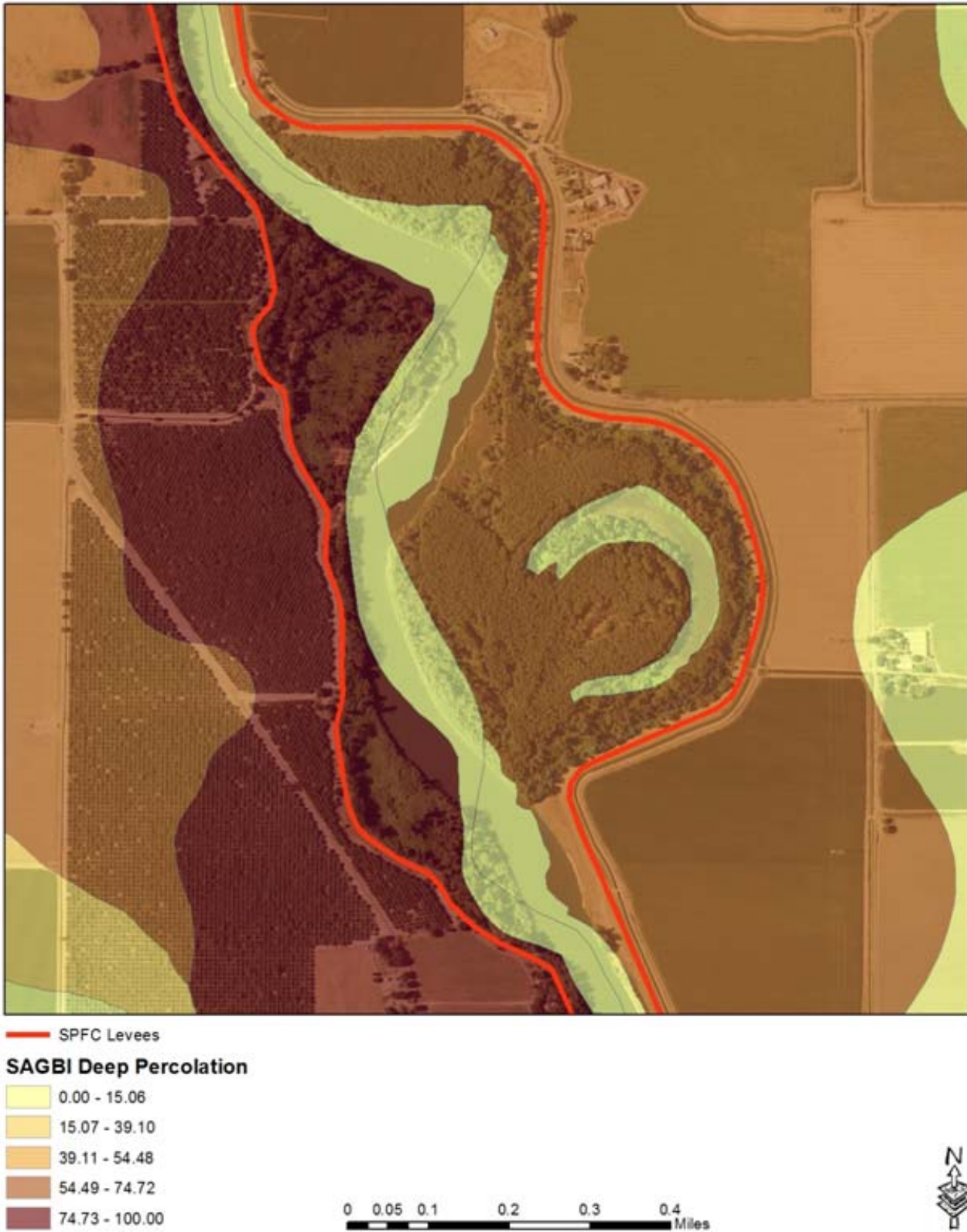
Figure 14. Map of deep percolation areas based on UC Davis’ Soil Agricultural Groundwater Banking Index (SAGBI)
