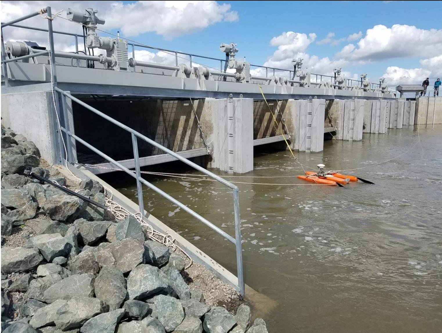
Notes: flow measurement at Wallace Weir showing typical Acoustic Doppler Current Profiler in a tethered trimaran.
