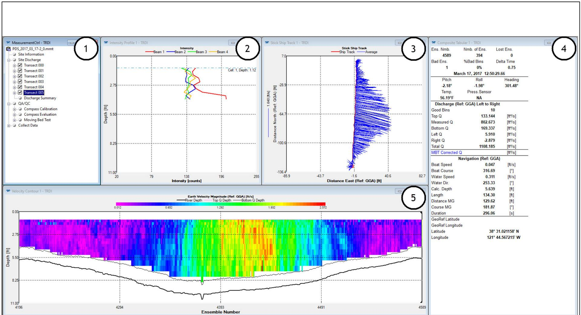
Notes: Winriver II output showing Acoustic Doppler Current Profiler (1) transect number, (2) beam intensity, (3) flow direction, (4) flow summary, and (5) velocity distribution.
