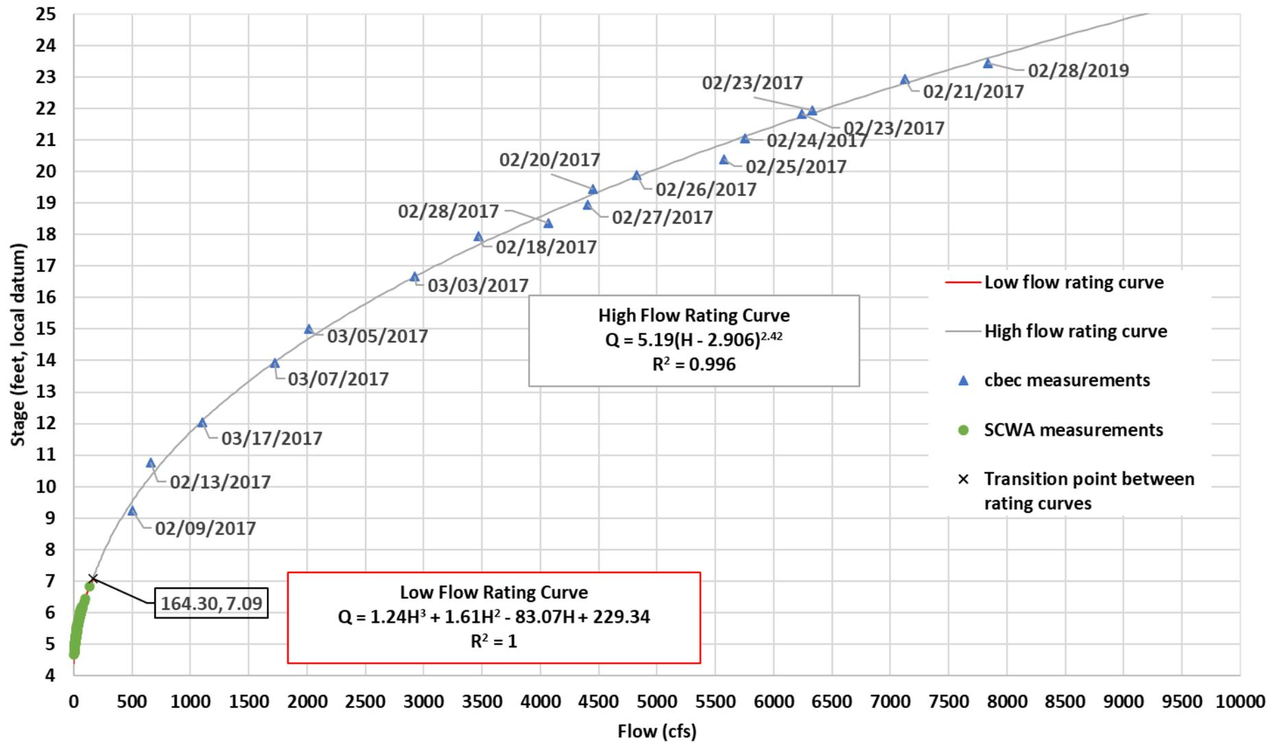
Notes: the low flow curve is based on Solano County Water Agency (SCWA) published rating curve. The high flow rating curve is based on this study using measured flows and SCWA published stage.
