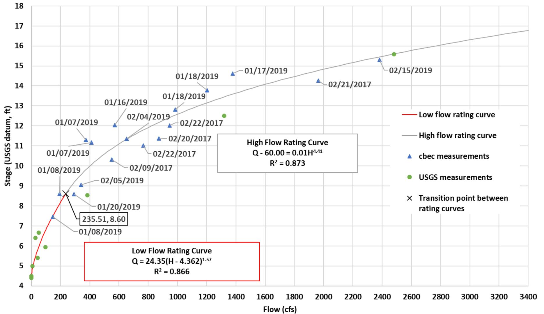
Notes: the low flow curve is based on USGS published data. The high flow rating curve is based on this study using measured flows and Yolo County Flood Control and Water Conservation District published stage.
