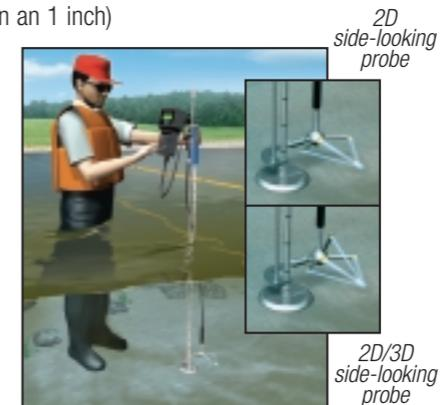
Example of typical stance and technique when using the FlowTracker
