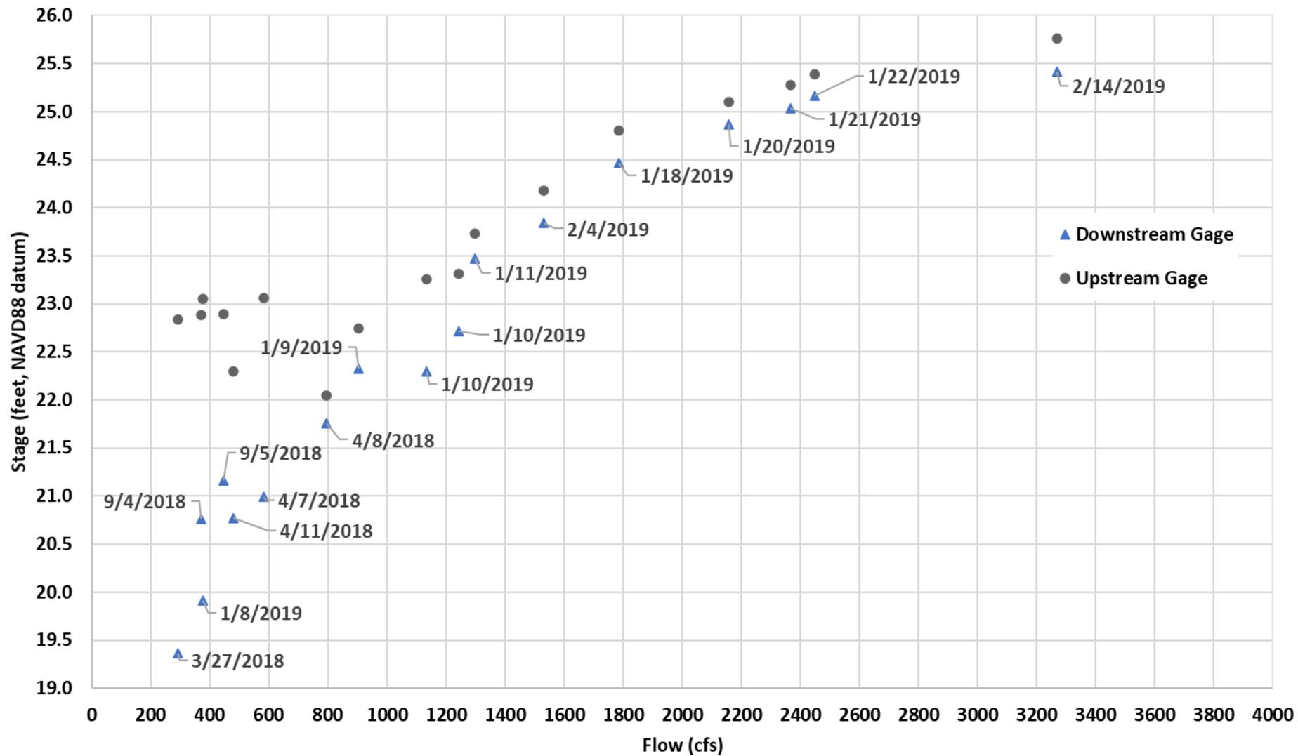
Notes: Stage and Flow correlation between measured flow and cbec redundant water level gages near Wallace Weir
