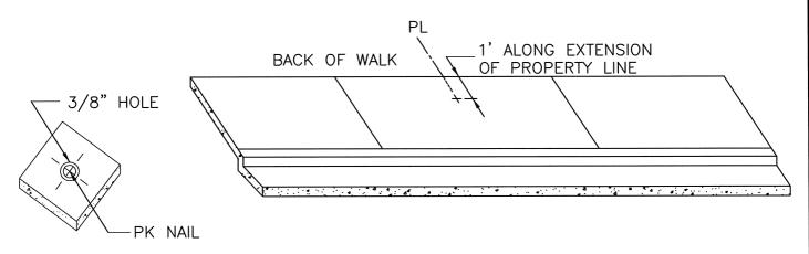
DRILL 3/8" DIAMETER HOLE FILL WITH EPOXY AND INSTALL 3/4" LONG PK NAIL SO TOP OF HEAD IS FLUSH WITH WALK.
