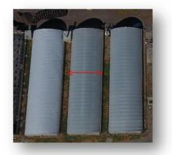
**Greenhouse/Hoop-House Width Definition:** The red line in the picture above represents how the width of a greenhouse/hoop-house is measured.
