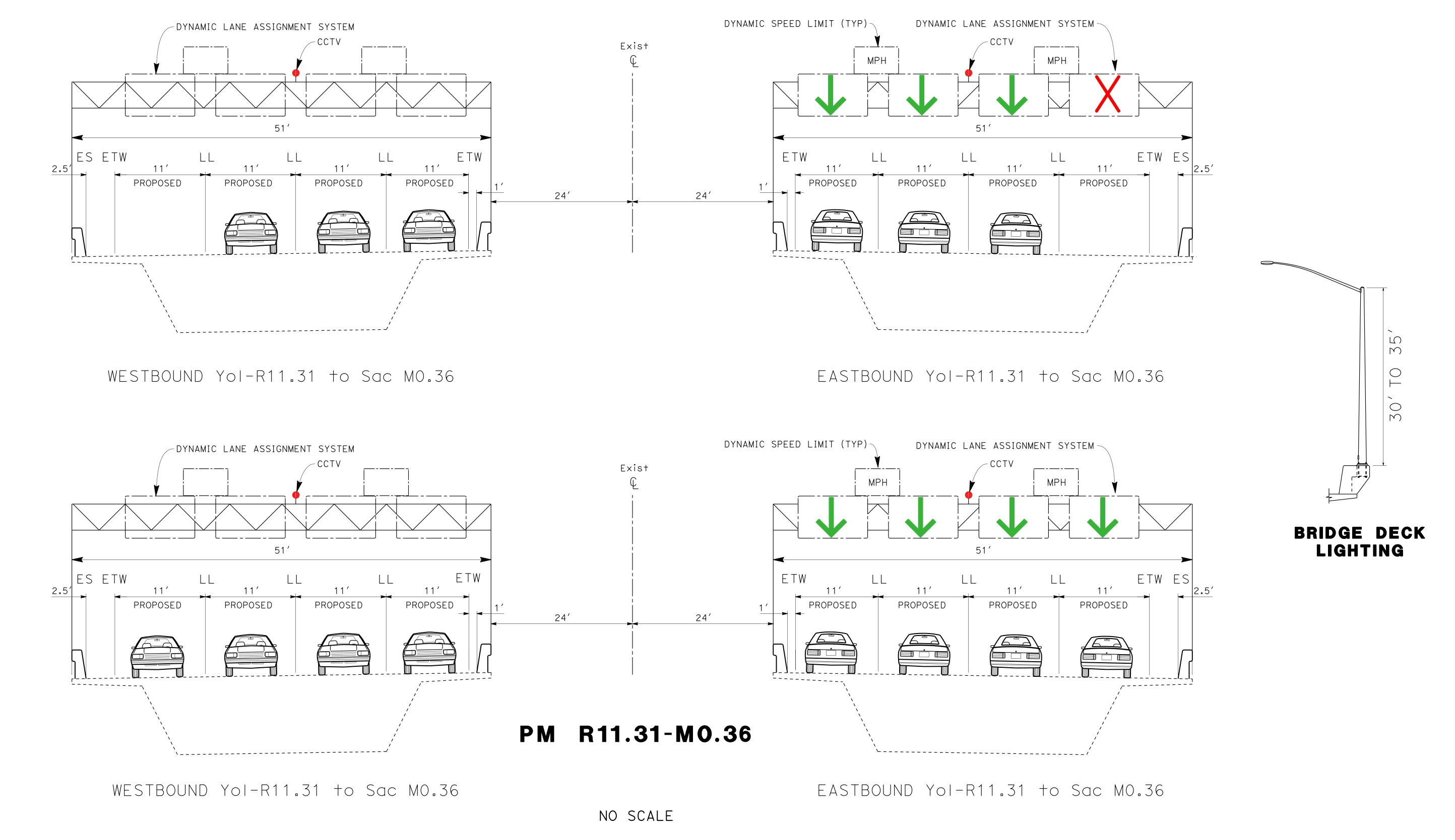
DLA OVERHEAD STRUCTURE WITH CLOSED CIRCUIT TELEVISION (CCTV) SYSTEM AND DYNAMIC SPEED LIMIT SIGNS LIGHTING ADDED TO BRIDGE DECK MAY RESULT IN LIGHT BEING DISPERSED BELOW THE BRIDGE TO THE SURROUNDING AREA
