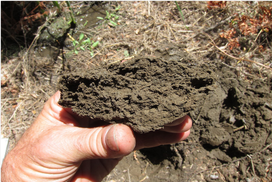
Photo 8. Soil from test pit at DP-2, with no redoximorphic features at all (100 percent 2.5YR 3/2).
