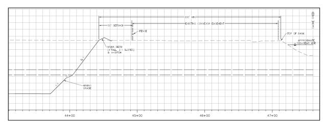
As shown above, the proposed mining slope inclinations are \(^3\)4:1 in the upper slope, 2:1 near the ground water level transition and 1:1 below groundwater. These slope inclinations and the overall mining depth are the same as previously proposed with the Moore Canal being relocated north. The only change is that the proposed mining will now be within 200 feet of the top of bank of Cache Creek instead of 300 feet.
