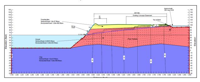
As shown above, similar to our previous analysis, the seepage front does not intercept the proposed north mining slope at an elevation higher than the average seasonal high groundwater condition, even when sustained indefinitely. Therefore, we do not expect an adverse seepage condition that would impact slope stability.
