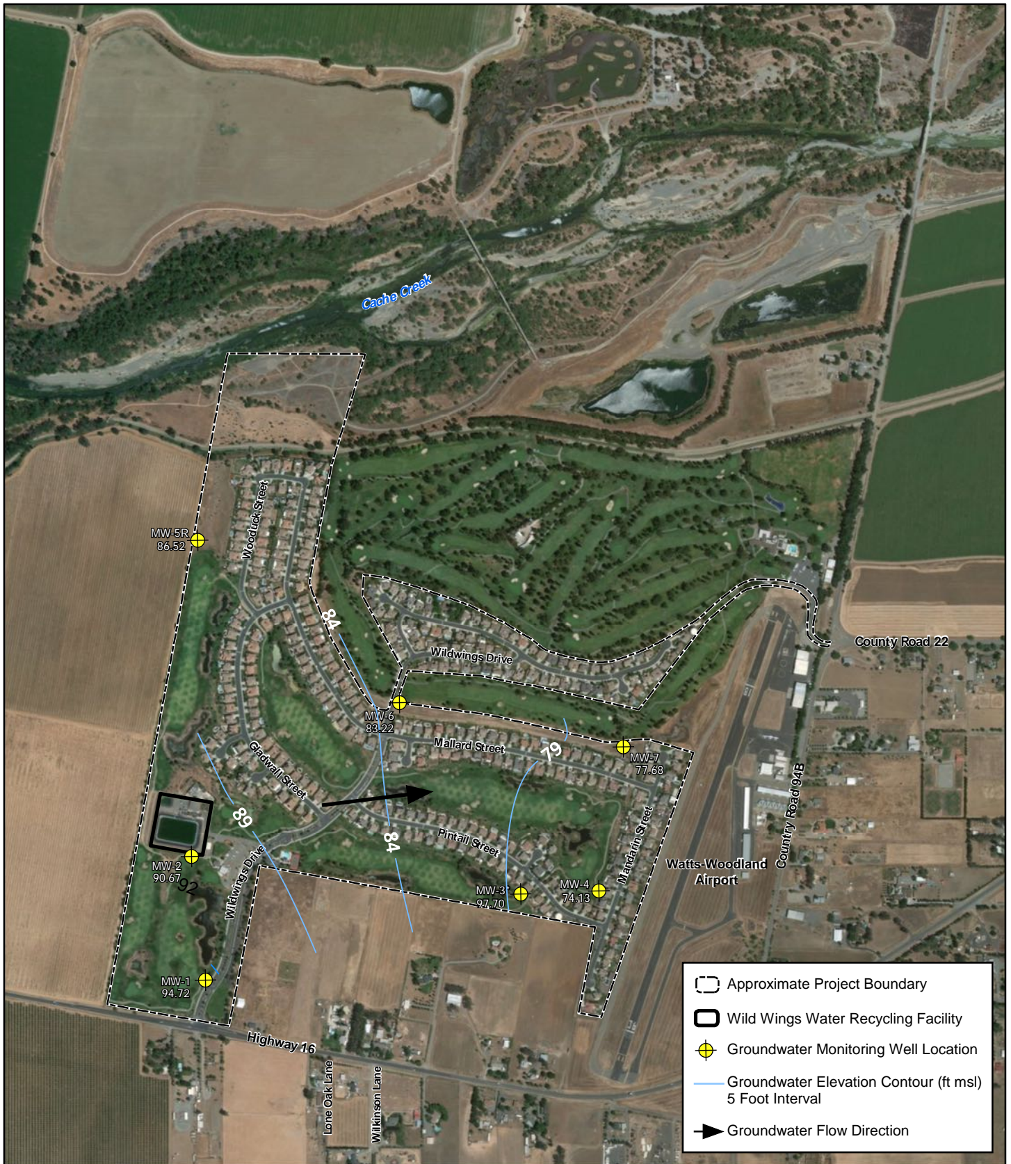
Figure 2 Groundwater Elevation Contours
