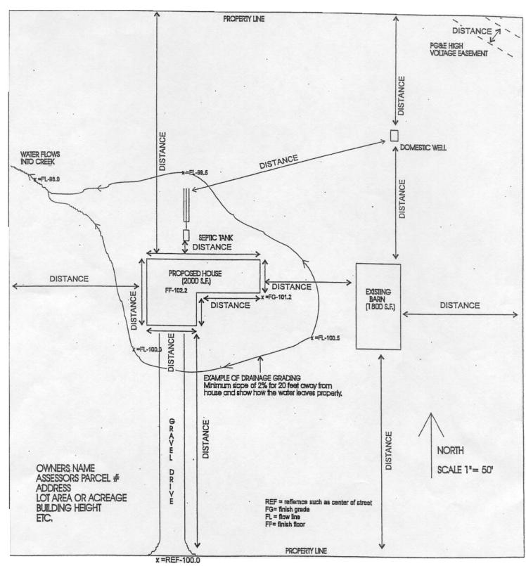
(without a true survey a point is picked as the reference elevation as the center of the street)
