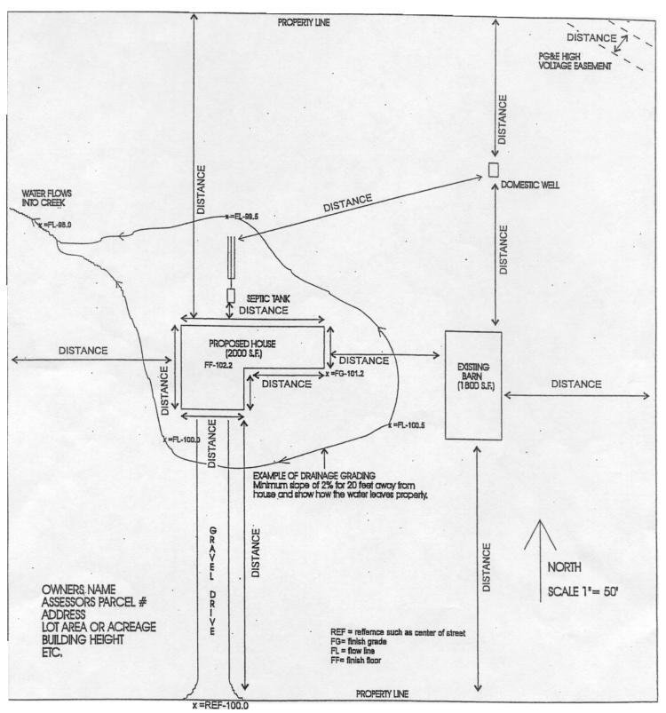
(without a true survey a point is picked as the reference elevation the center of the street)
