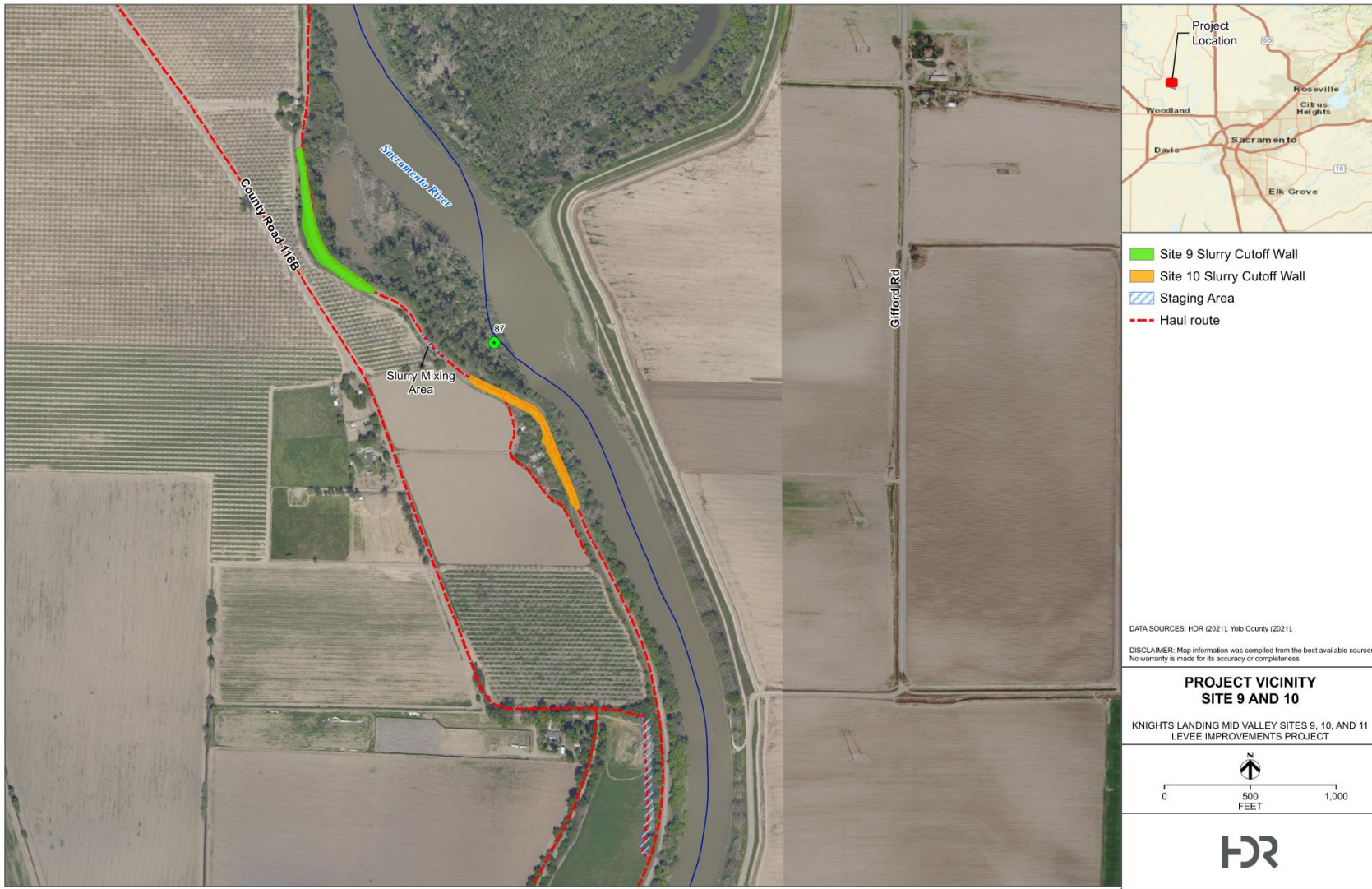
Figure 2.2-1. Mid-Valley Levee Reconstruction Sites 9 and 10 Project Area
