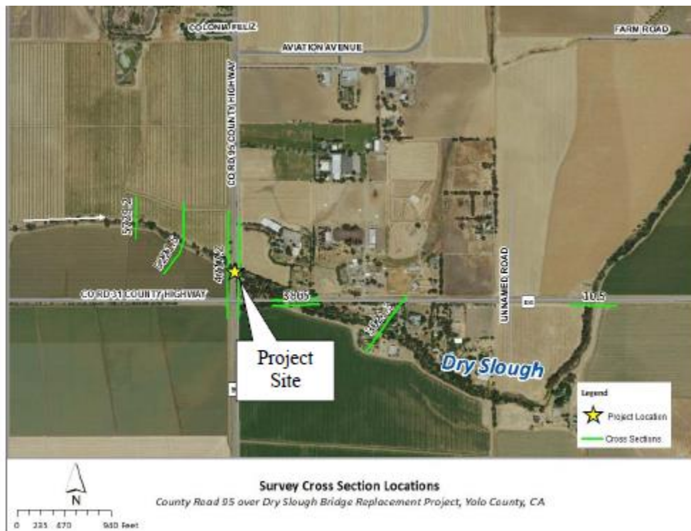
Figure 17: HEC-RAS 1D Cross Sections
