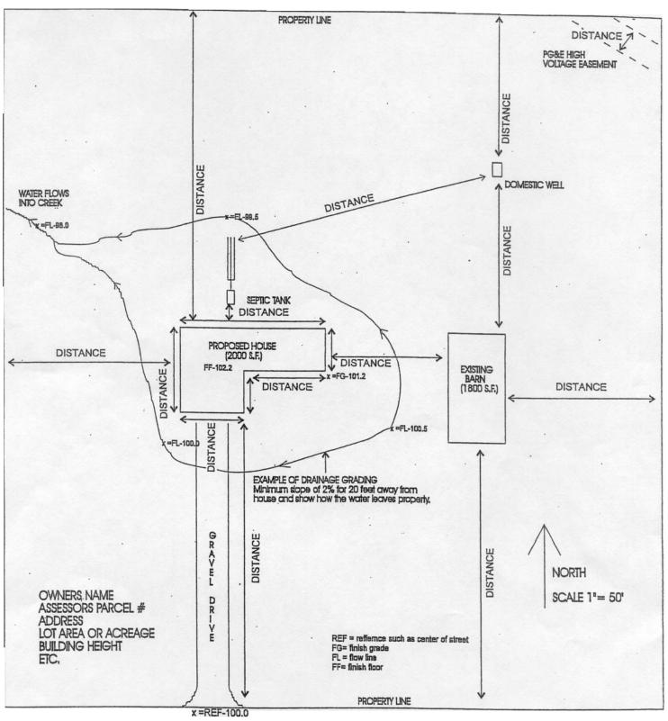
(without a true survey a point is picked as the reference elevation the center of the street)
