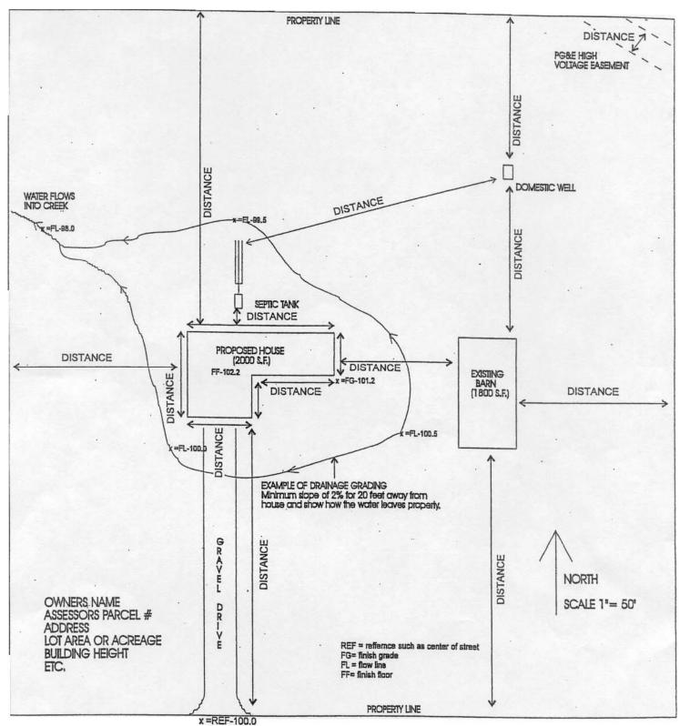
(without a true survey, a point is picked as the reference elevation C) DIM ROAD  $\underline{\text{such}}$  as the center of the street)
