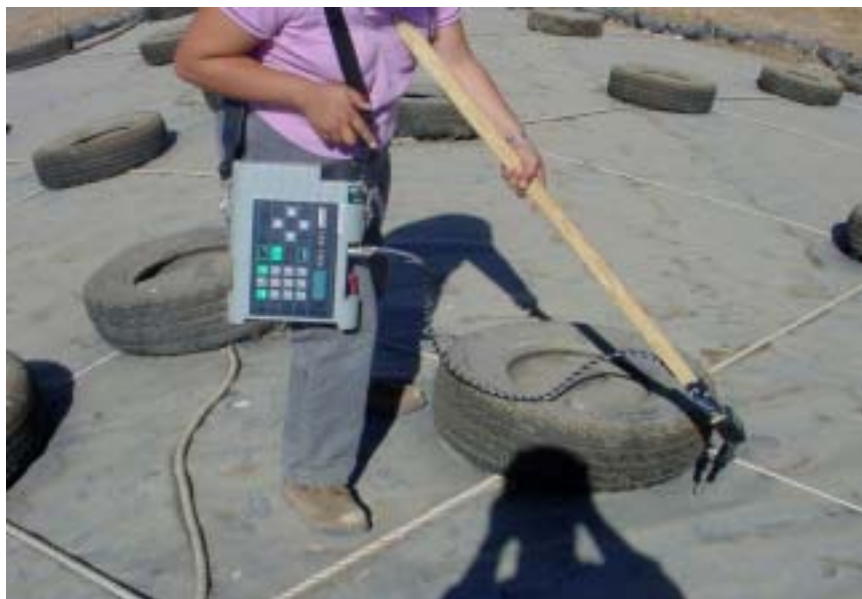
Image 3-6. Surface emission monitoring with the TVA 1000.
