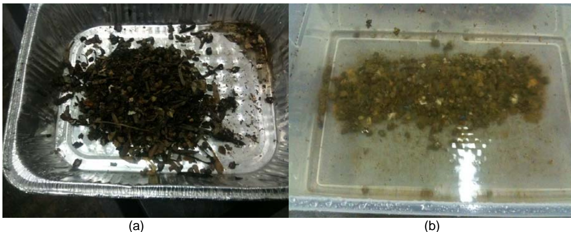
Figure 12: Light (a) and heavy fraction (b) using separation in a water bath.
