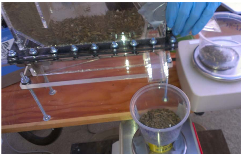
Figure 10: Fluidized-bed separator. Light material travels to the upper right, heavy material to the right and front.
