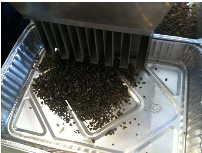
Figure 2: Riffle splitter for splitting a sample into a smaller sub sample. Samples were split four times in half to obtain approximately a 16th of the amount of the original sample.
