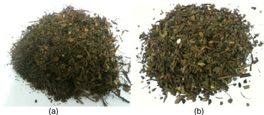
Figure 11: Light (a) and heavy (b) fraction of #8+ class after separation in fluidized-bed
