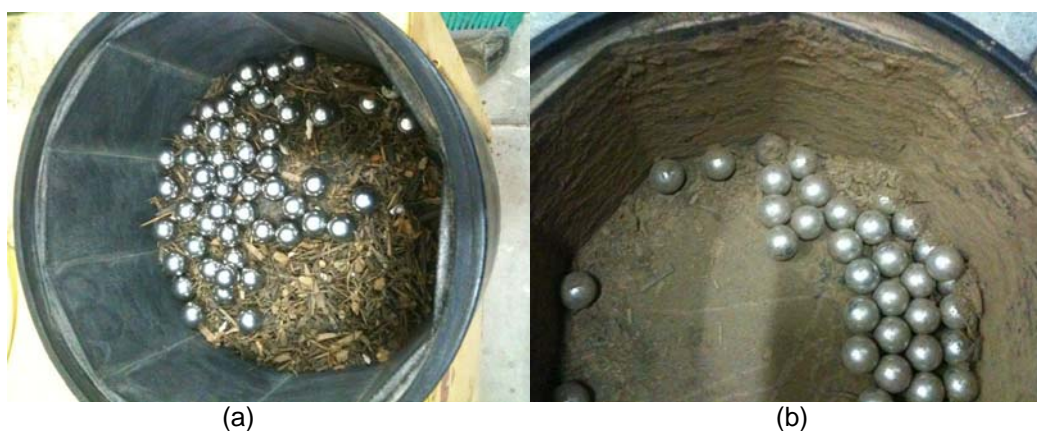
Figure 13: Light fraction of #8+ size class before (a) and after (b) grinding in ball mill
