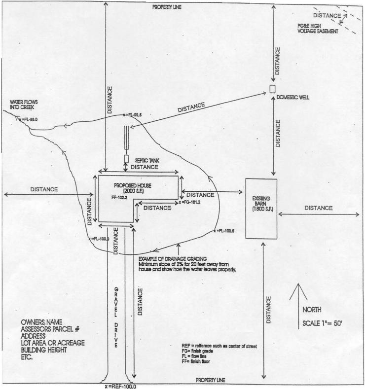
(without a true survey, a point is picked as the reference elevation C) DIM ROAD <u>such</u> as the center of the street)
