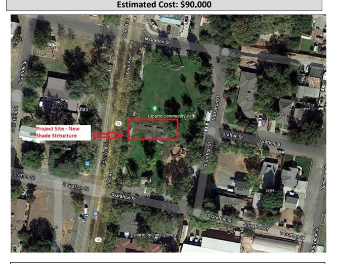
**Scope of Work:** Purchase and install a permanent shade structure to be placed over the existing picnic and BBQ area at Esparto Community Park. The structure's footprint will be approximately 40 feet x 24 feet made from fabric UV rated material.
