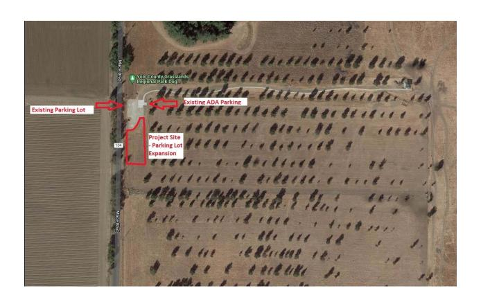
**Scope of Work:** Expand existing compacted gravel lot South of the existing parking lot. Will expand parking stalls by 30. No ADA additions are required.
