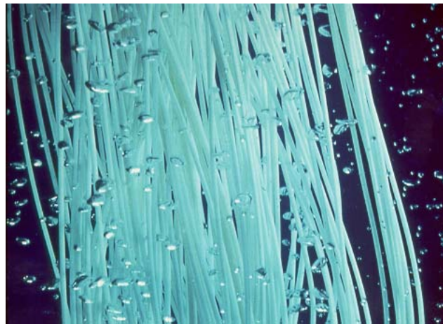
Figure 2. Hollow-fiber membranes (Image from GE/Zenon)
