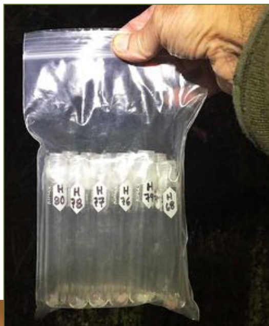
A9. Set of small muscle samples; fish released, vs. standard method that sacrifices fish
