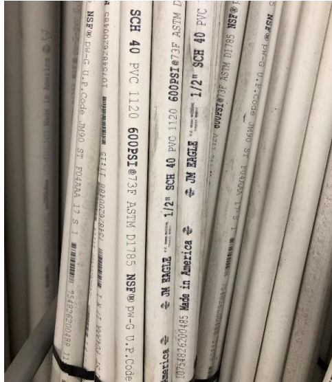
Potable white PVC line with NSF label
