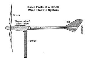
In typical residential applications, a home is served simultaneously by the wind energy system, and a local utility. If the wind speed is below "cut-in speed" (7-10 miles per hour), all of the needed electricity is obtained from the utility. As wind speed increases, the system's electrical output increases, and the amount of power from the utility is proportionately decreased. When the system produces more electricity than the house needs, the extra power may be sold to the utility.
