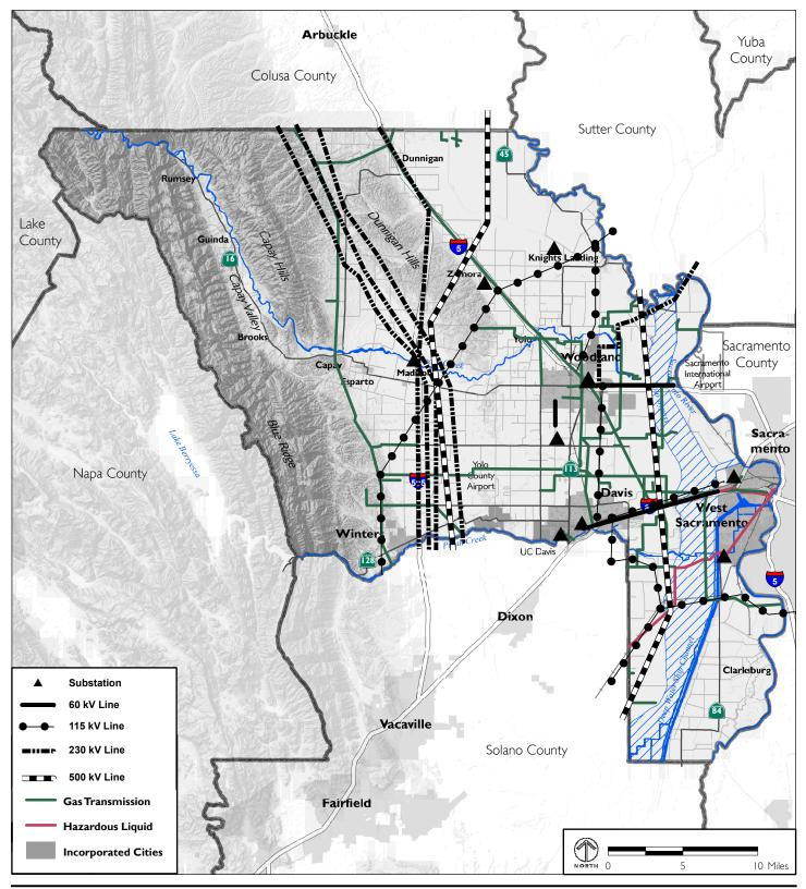
Source: Transmission Line Element, Yolo County General Plan, 1990; National Pipeline Mapping System, Pipeline and Hazardous Materials Safety Administration. Note: Gas transmission and hazardous liquid pipelines were roughly estimated from data obtained from the Pipeline and Hazardous Materials Safety Administration.
